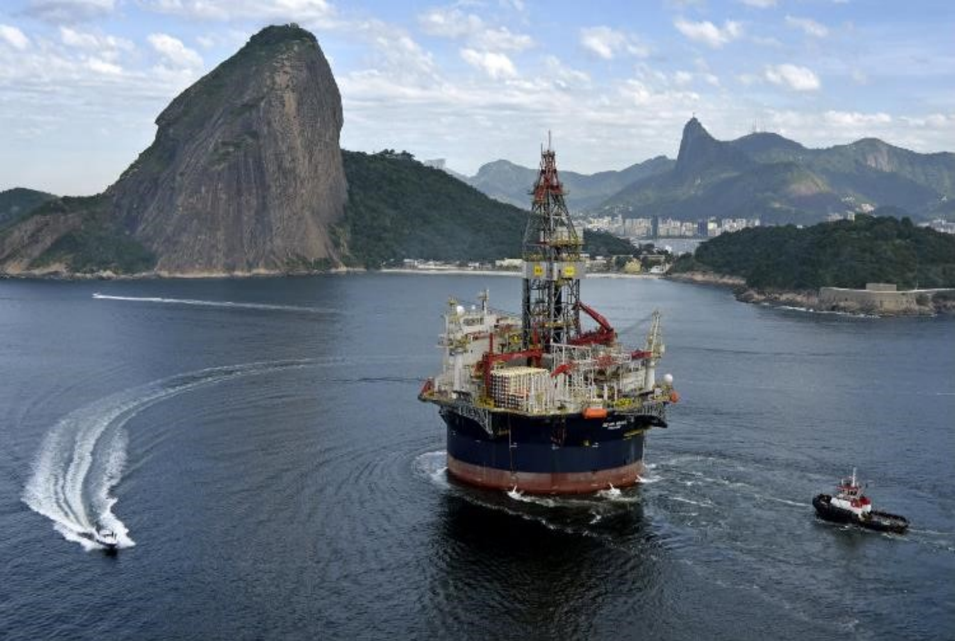
A new design of deepwater drilling rig based on the success of Spar production platforms
