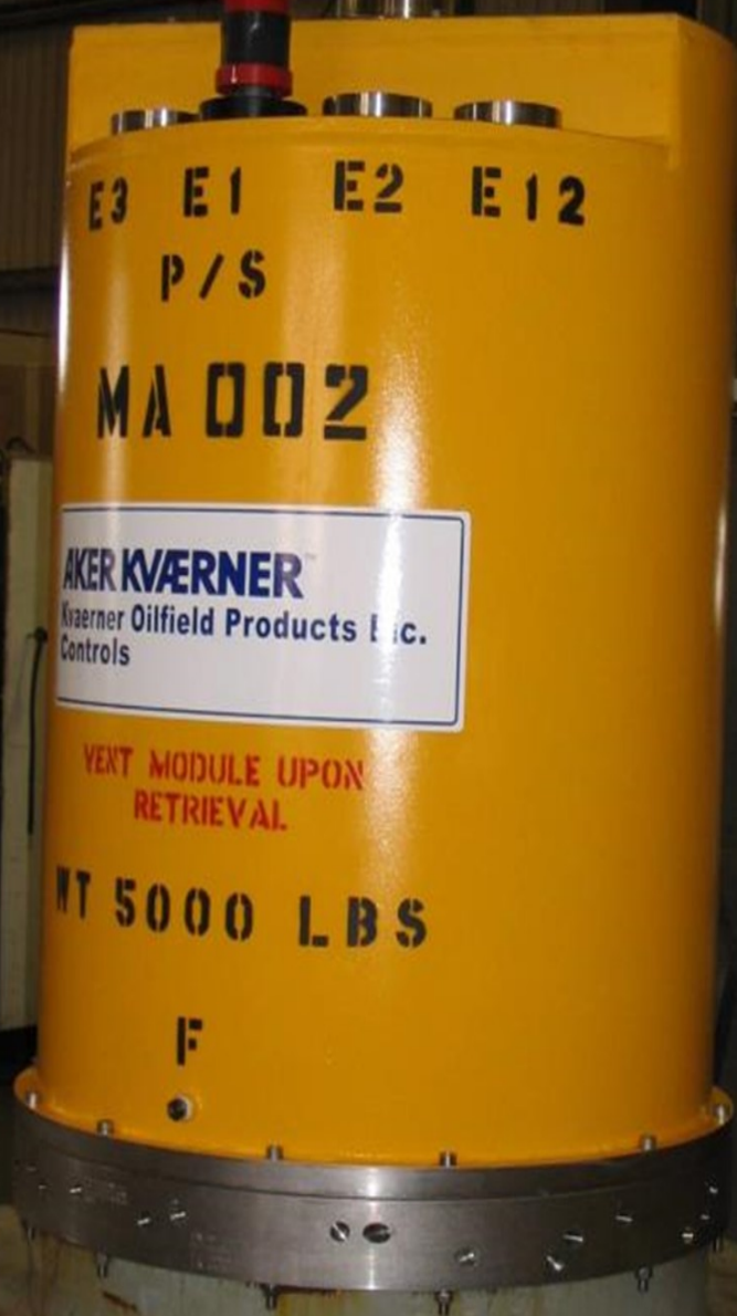
Subsea Control Module C
