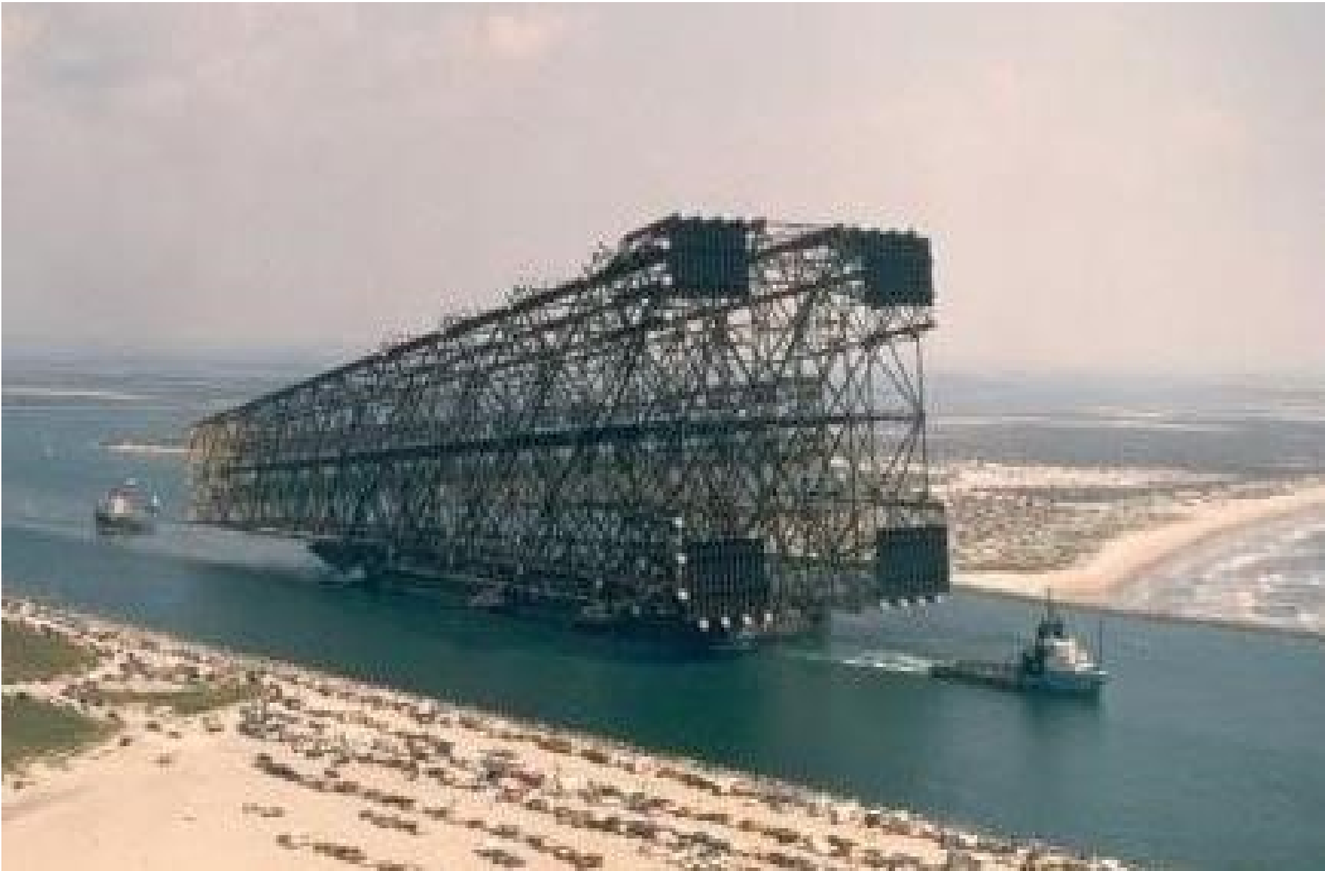
Bullwinkle: GOM, 1066' W.D. About as deep as you can go with gravity
