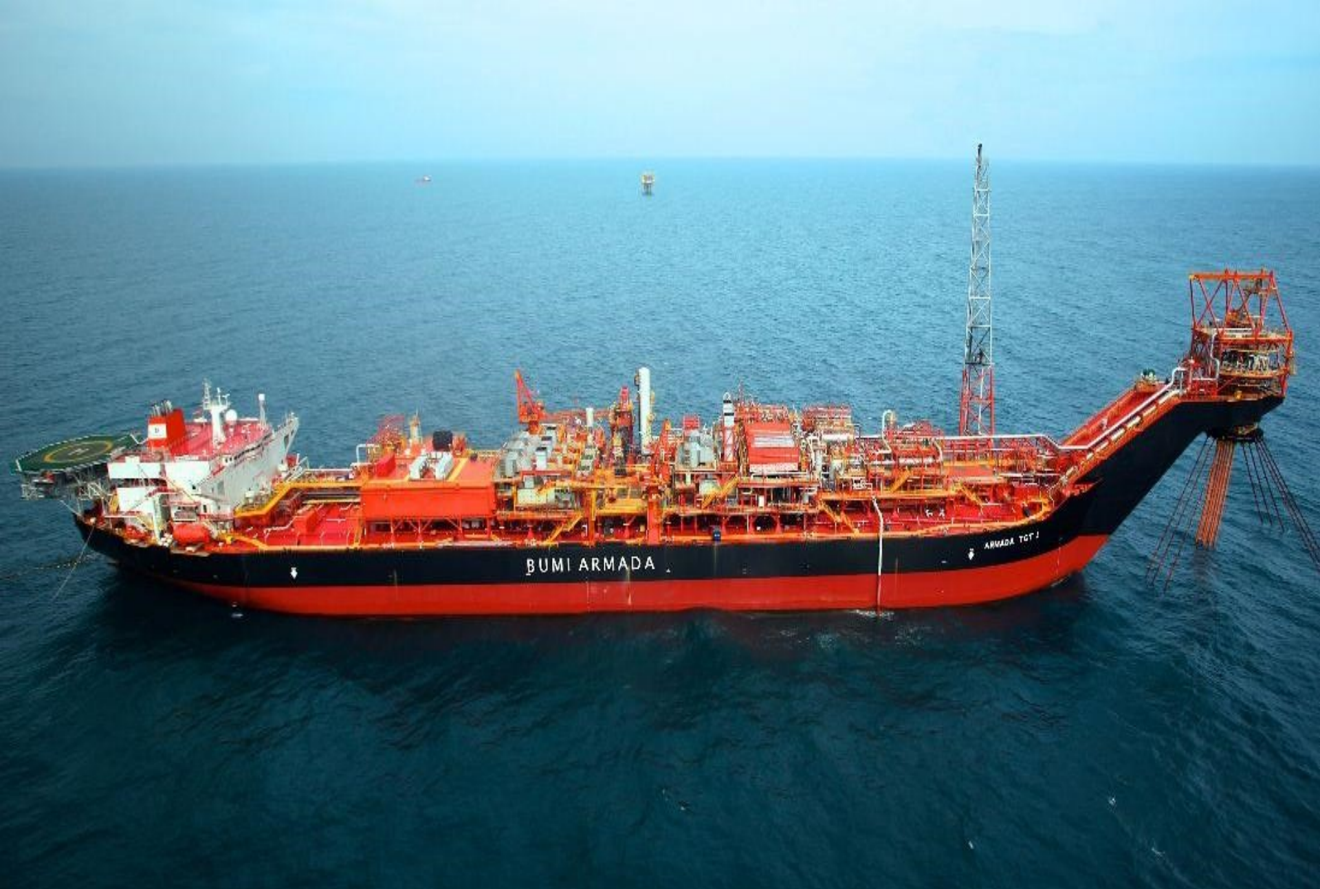
External turret FPSO
