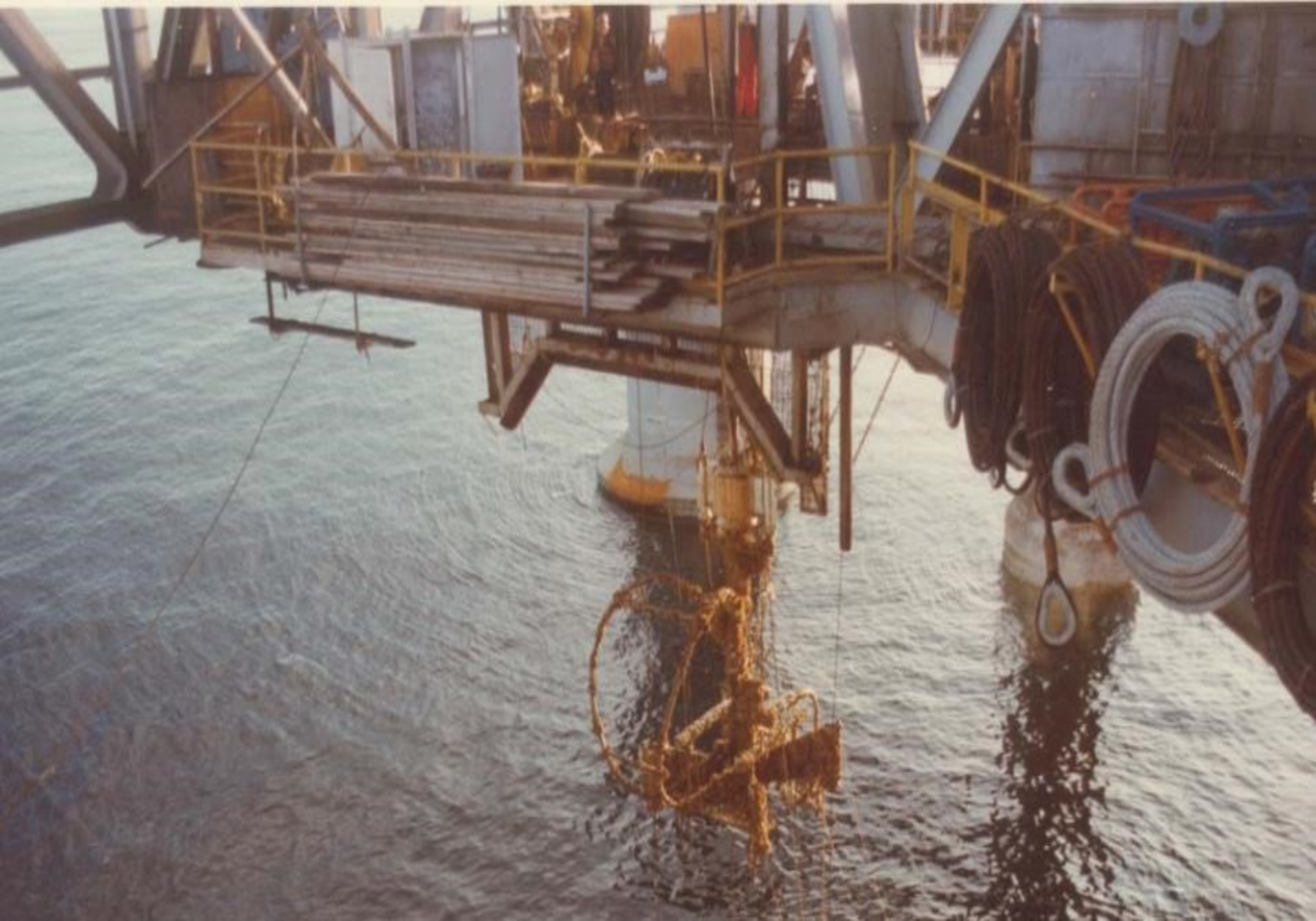
The world's first subsea tree being retrieved. 1961-1995
